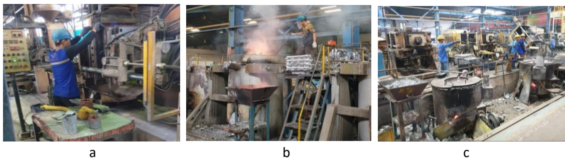
Figure 4 a. Sand Core Making Process, b. Melting of Metal, c. Casting Process
