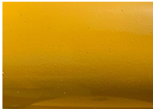
Gambar 5. (a) Cacat Mottling ; (b) Cacat Dust Spray
